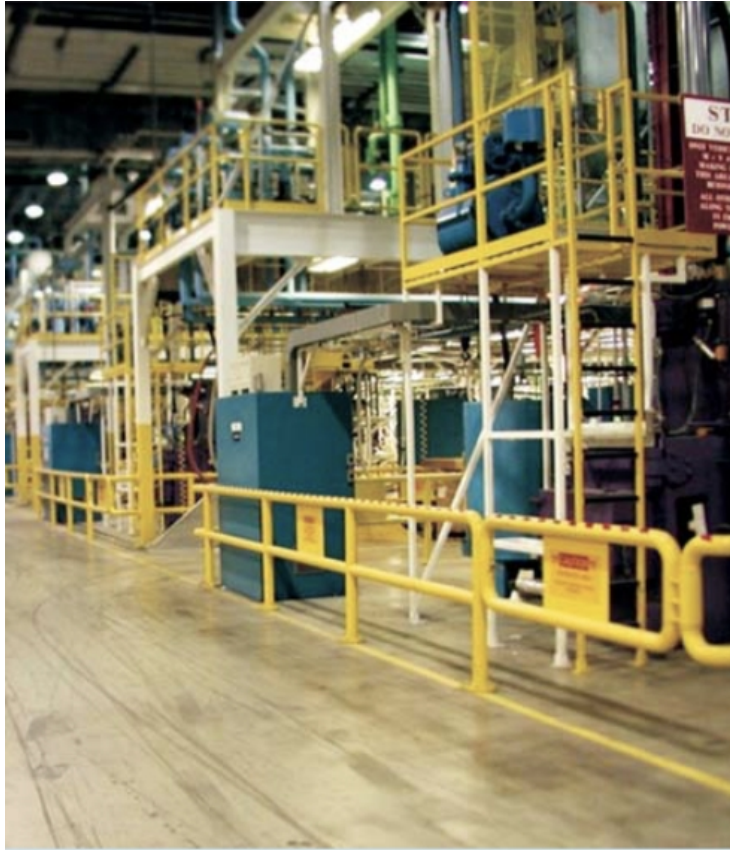
Figure 2. A typical electron-beam processing facility, employing 10 large electron accelerators arrayed in a row of production stations. This facility produces shrink-wrap material. (Photo courtesy of Air Seal Corp, Duncan, SC.)
